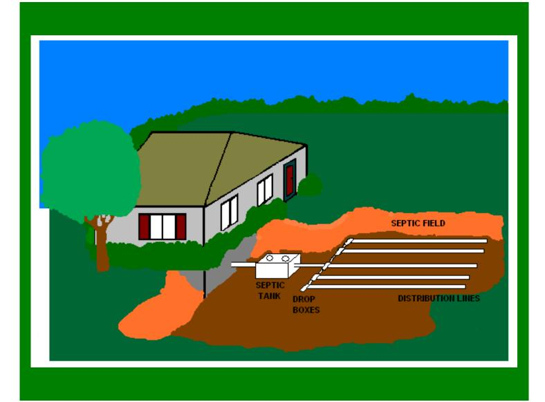
A septic system consists of a septic tank, drop boxes and a drainfield, all connected by pipes called header lines.
