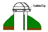
The well cap protects the well from environmental factors; surface water, vermin, fertilizers, herbicides, pets, etc. Maintain landscaping around the well casing and cap so rainwater will not collect around the well. Slope the ground away from the well and keep the well cap a minimum of 8" above the ground.
