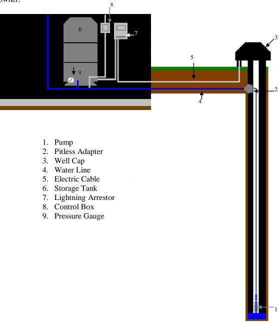
Your water well system draws water from the surrounding formations of rock into the well casing. The submersible pump pushes water through the drop pipe into the water line and into the storage tank. The water is distributed from the tank throughout the house as needed.
